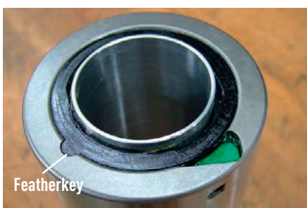
Fig. 10.3 Before assembly, ensure that the scrapers have been correctly housed
