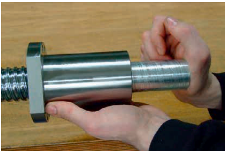
Fig. 10.5 Nut assembly with NBR/TPU seal on the shaft
