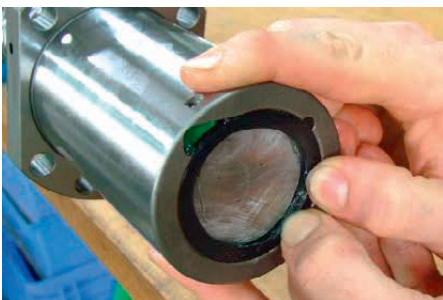
Fig. 10.6 Stop the NBR/TPU seal while slowly mounting the nut on the shaft
